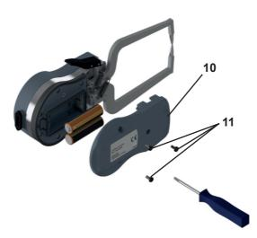
Insert the battery ensuring correct polarity!
